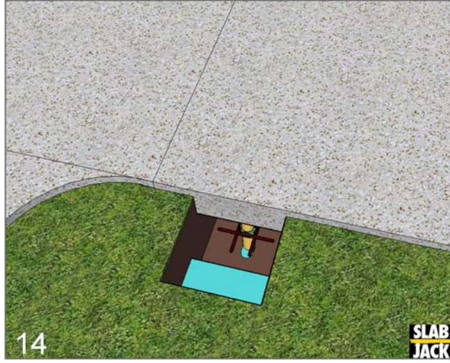
14 The LIGHT BLUE color shows the back fill soil to be placed to hold SlabJack and to minimize the amount of concrete that has to be poured.
