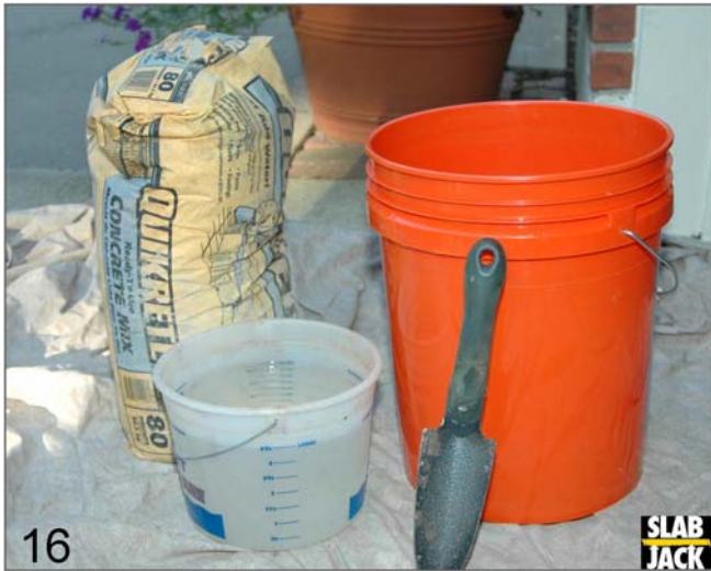
16 A 5 gallon bucket, a gallon bucket of water, an 80 pound bag of QUIKRETE and small mixing shovel. Place 4-5 inches of QK in 5 gal. bucket equals approximately 20 lbs. QK.
