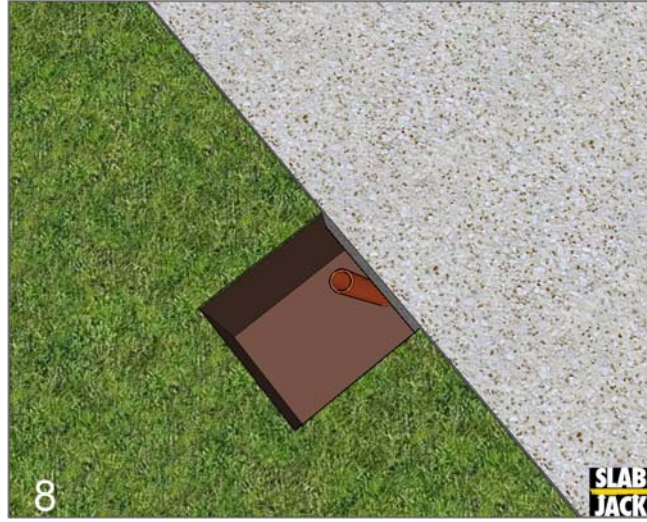
8 Surface view to show center line placement of PVC 1-1/2" schedule 40 x 2'-0 long to create a void to allow for SlabJack. (Purchase from local hardware store. Reused for each SlabJack placement.)
